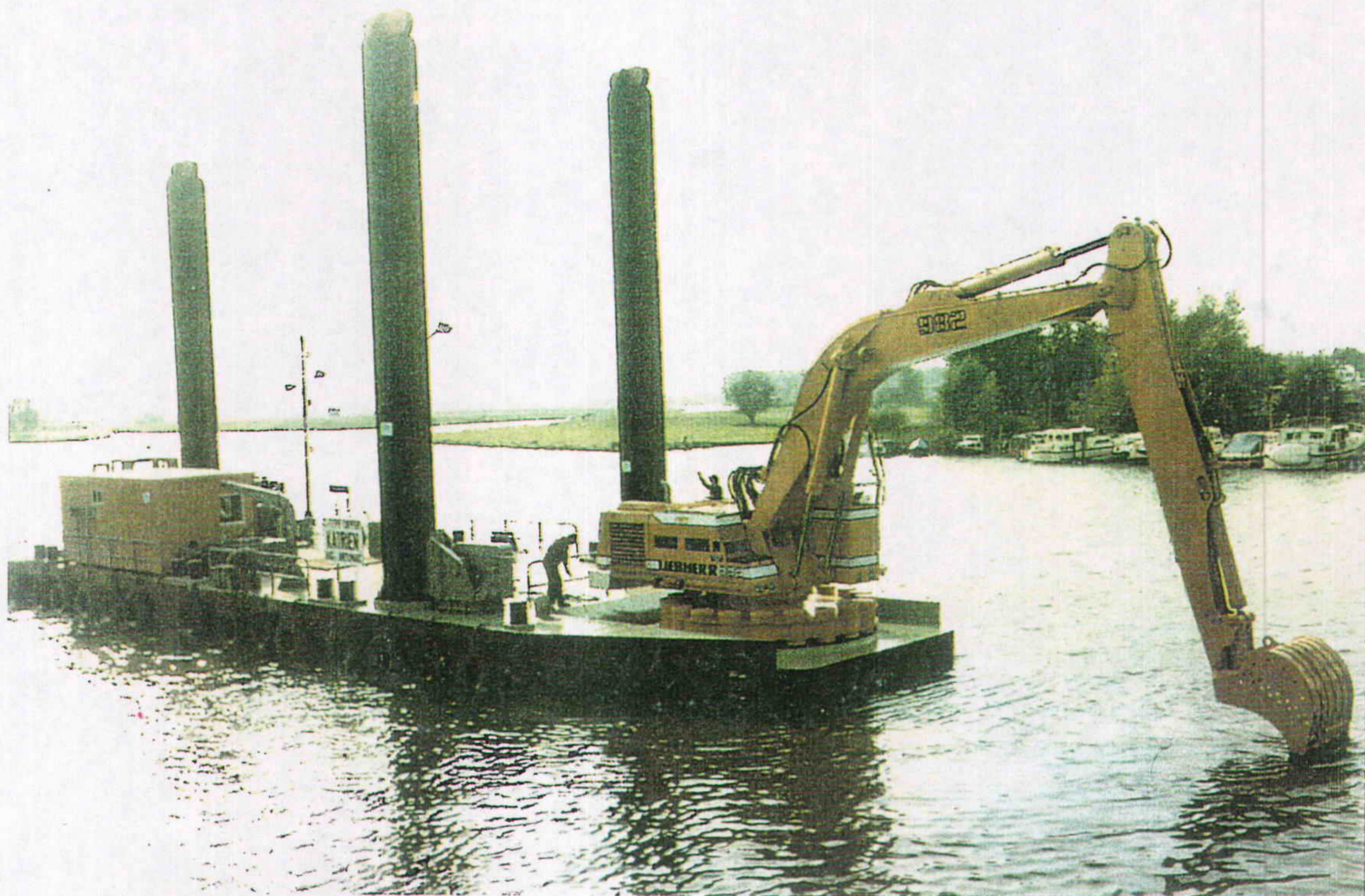
A typical C-type, protected waters dredger with round spuds. (Dipperdredger "Katrien" of Dredging International.)
